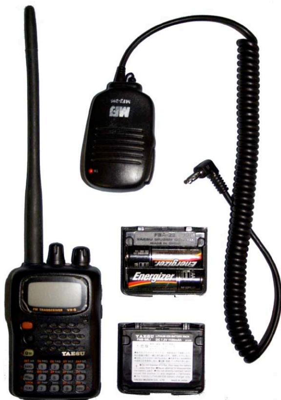
Typical miniature 5 Watt VHF / UHF Amateur 3-band handheld transceiver with rechargeable battery, emergency AA battery pack and external microphone.
