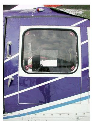
Each medium helicopter has a number of emergency exits. The main emergency exits for the passengers on medium Bell helicopters are often the doors or the large windows.
