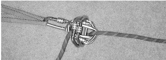
Locking carabiners are shown here, but they can be difficult to connect properly as the locking collars can get in the way of smooth assembly.
