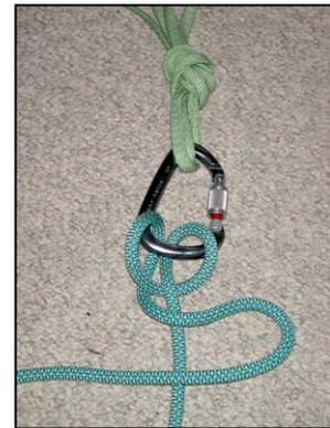
**←Step Five:** Clip this strand into the carabiner (orientation is critical here again) and you now have a properly oriented Monster. Lock the carabiner and you are ready to lower with the hand – behind – hand technique (milking the cow). You will notice that when the carabiner is loaded it stays oriented gate out and the line you are controlling exits the carabiner on your side while the loaded line is centered. Perfect.
