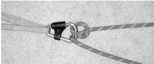
**Step One:** Hold the load on the Munter Hitch tightly during the entire process and **DO NOT** let go of the braking hand, even for an instant.
