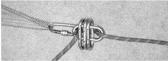
For a large single person load an additional carabiner can be added to increase the friction. Oval carabiners work well for constructing these brakes.
