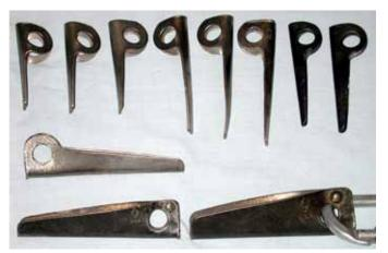
Angle pitons are made by folding a sheet of metal in a "U", "V" or "Z" shape. By using folded sheets of metal instead of a solid piece of metal the weight of a piton can be reduced in the larger size ranges.
