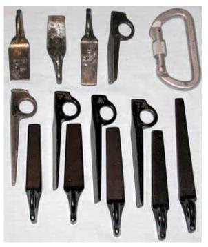
The common "Lost Arrow<sup>™</sup>" design of piton is a type of horizontal blade piton. The thickness of these pitons varies from just slightly thicker than a knifeblade to almost 1cm thick near the eye.
