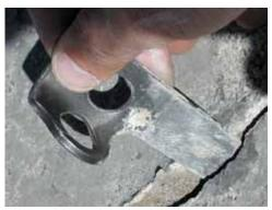
Select the appropriate size and type of piton for the crack. Orient the eye of the piton in the anticipated direction of pull (most often down). Ideally in a clean crack the piton should go in and be snug when it is about 1/2 to 2/3 of the way in. If the crack is filled with dirt or mud, attempt to clean it as well as practical in a timely manner.
