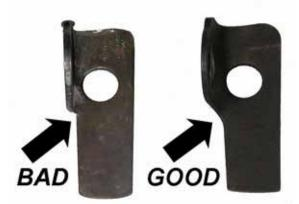
In recent years there have been some poorly manufactured knifeblade pitons on the market. In metal manufacturing any sharp or square inside corner can result in stress fractures or cracks and under load these cracks can propagate. The piton can then tear and fail.
