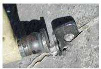
piton begins to loosen. Once it is loose, all that is often required is tapping it lightly into the center and removing it by hand.
