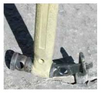
Truly stubborn blade or angle pitons can be removed by prying on the eye if your hammer has a long thin nose which is designed for this purpose.
