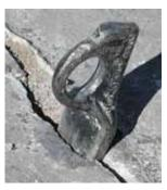
If the piton doesn't go in all the way to the eye, it is best to remove it and use a more appropriate sized piton or place the
