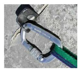
Once your piton has been tested, all that remains is to clip into the piece and appropriately attach the rope or build the rest of the anchor. For anchor building considerations see the article "Anchors in Earnest". Once a sling or rope is attached some people prefer to conduct a final test by tugging on the sling in all directions, including straight out, to be sure the placement is solid.
