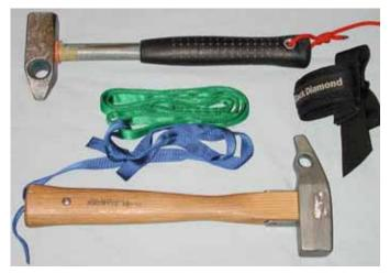
A heavier hammer with a hefty shaft is best for rapid driving of pitons with less hammer vibration and fatigue. If a lot pitons are going to be driven, the choice is for a beefy hammer typically with a wooden shaft or sometimes a metal shaft and rubber grip. Having a flat anvil on one end for driving the piton and a somewhat pointy nose on the other for aiding in piton removal are common useful design features. Some
