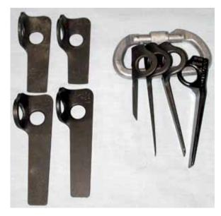
**Blade pitons** vary in thickness from the thinnest designs which are barely as thick as a knife blade to the thicker end of the spectrum where pitons are perhaps one centimeter (just less than half an inch) thick.
