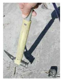
Once you have driven the piton in until the eye touches the rock you should still do a final check of the placement. Visually inspect that no cracks developed, there was no shattering of the surrounding rock or widening of the crack in which the piton was placed.
