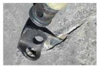
Removing blade pitons is simply a matter of pounding the piton back and forth as far as it will go. Continue this action with repeated blows in each direction until the
