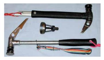
When pitons are going to be used only occasionally and in climbing situations where weight is a consideration, climbers will often opt for a lighter hammer. Some modern lightweight hammers have a hollow plastic shaft for weight reduction. On alpine climbs some will use a multi-purpose tool that can be used as both an ice hammer and rock hammer. The hammers
