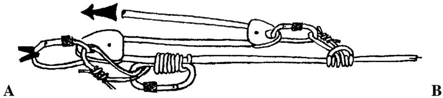
3:1 simple system with Bachmann Hitch minded by a pulley
