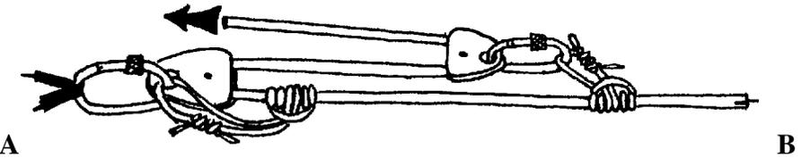
3:1 simple system with Prusik Hitch minded by a pulley
