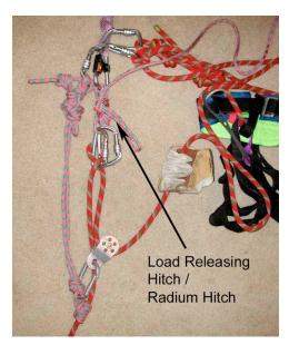
Advanced Procedure: Attach a Load Releasing Hitch if required. In this case a Radium release Hitch 2:1 has been used. See the articles "Radium Release Hitch 2:1 for Improvised Rescue" and "Load Releasing Hitches" for further information.
