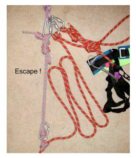
**Step Ten**: Remove the belay device from the rope and you have fully escaped the system. The rope is now attached to the anchor via the Prusik cord and is backed up by a knot on the main line. At this point you must decide which rescue procedure must be performed. The sequence that follows assumes that you will be raising the fallen climber with a pulley system although this may not be your first choice in any given situation.
