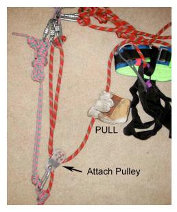
**Step Twelve**: Attach a pulley to the slack rope and attach the pulley to the carabiner previously placed next to the Prusik Hitch on the rope. If no pulley is available attach the rope directly into the carabiner with a resultant loss in efficiency. For a discussion of pulley use in improvised rescue, see the article "*Pulleys and the 3:1 System*."
