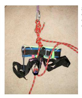
**Step One**: *Prepare to Tie-Off the Belay*. Orient yourself directly in line with the fallen climber so that a minimum of effort is required to keep yourself in balance and you can concentrate on the knots and ropework.
