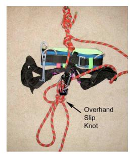
**Step Four**: Using just a single strand of rope, tie an overhand slip knot directly in front of the belay device so that any additional load that comes on the belay device continues to tighten the knot. (Practice this under supervision so that it becomes automatic *before* you have to use it in a real situation!)
